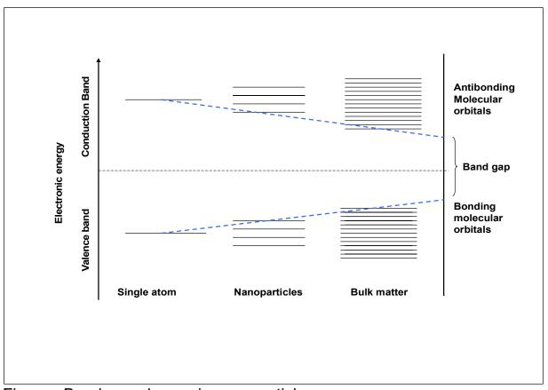
Figure: Band gap change in nanoparticles
